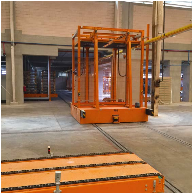
The MSK shuttle car allows quiet and automatic pallet transport.
