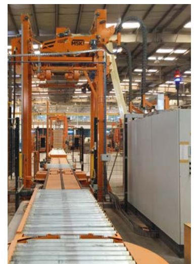
The MSK Multitech shrink hood wrapping machine packages glass pallets with a robust protective UV film.
