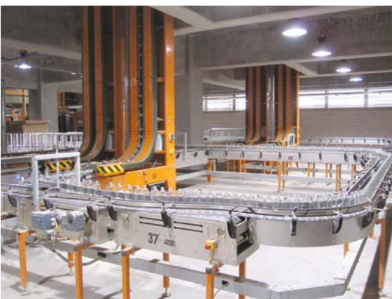
MSK bottle conveyors transport the glass containers to the palletisers.
