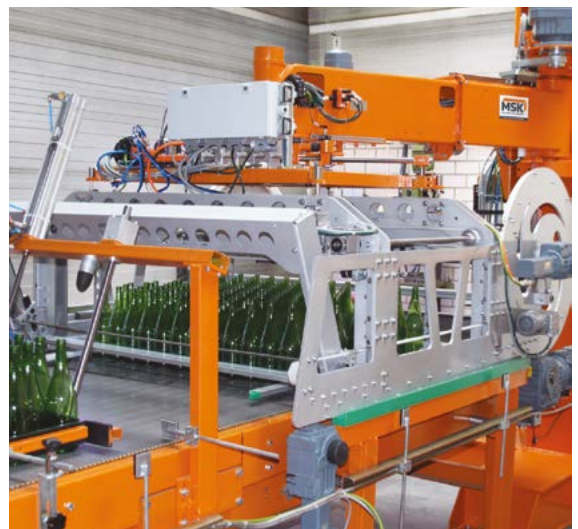
The universal palletiser from MSK flexibly processes a wide variety of bottles.
